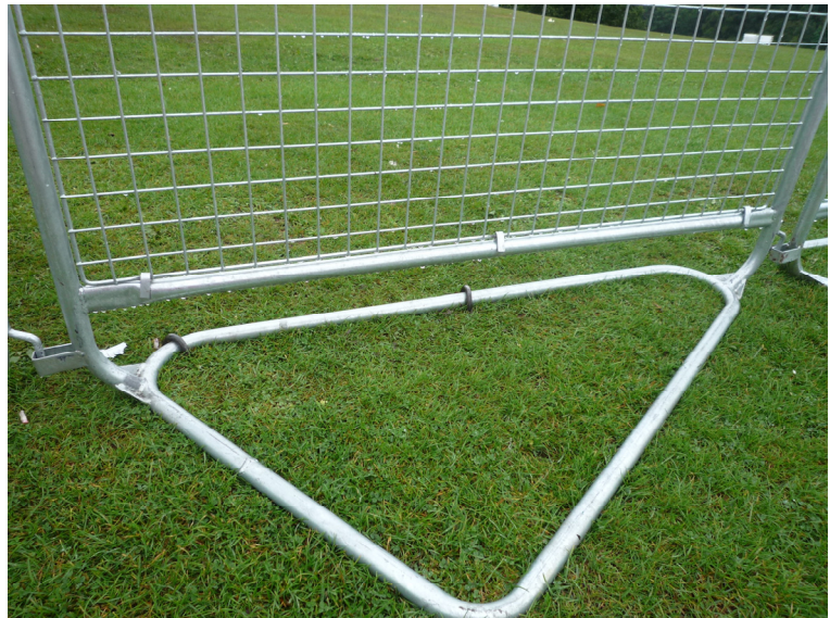
Fig. 23-3 - A different foot design, intended to resist a modest degree of pressure. Note the pinning of the foot to further stabilize the barrier. Photo courtesy of The Event Safety Shop, LTD.
