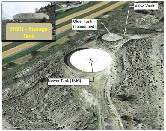
Figure 2-35: Forsyth Hill 1 MG Water Storage Tank
