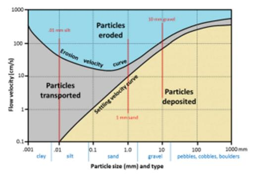
Figure 4-4 Intake Vel vs Particles Carried
