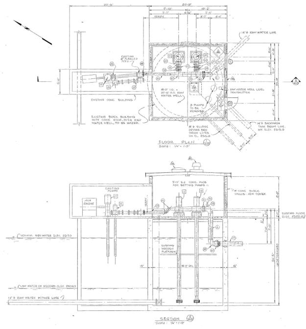
Figure 2-28: Intake structure plan and profile
