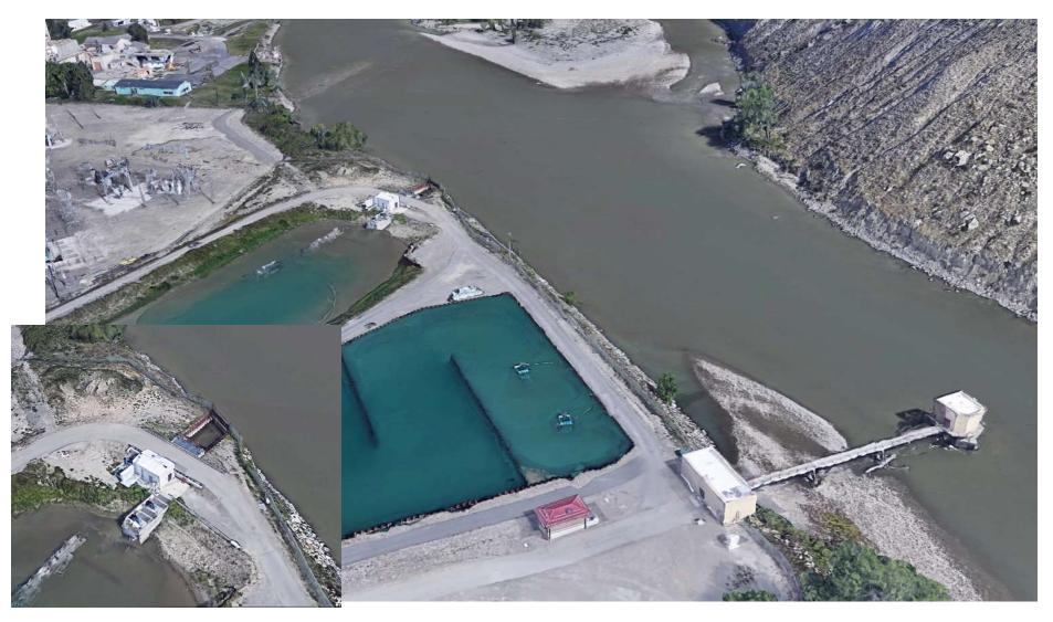
Billings' Two Intakes: Side Channel System (see inset) and In-River Crib & Barrel Structure (lower right)
